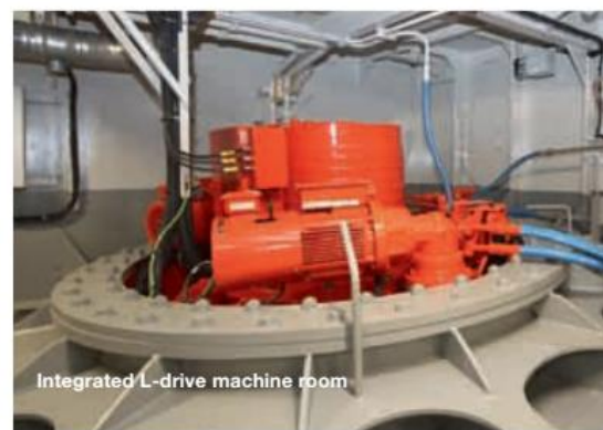
Damen's Volt Processor during sea trials with the Integrated L-Drive.
